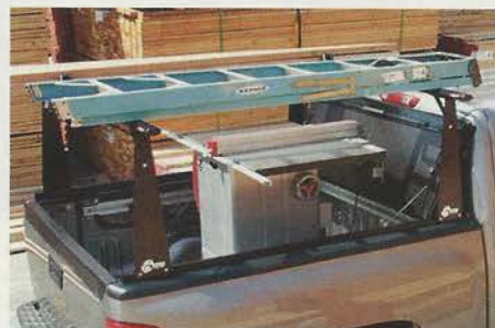
BAK Flip CS incorporates a 500 lb rack to load long objects overhead
